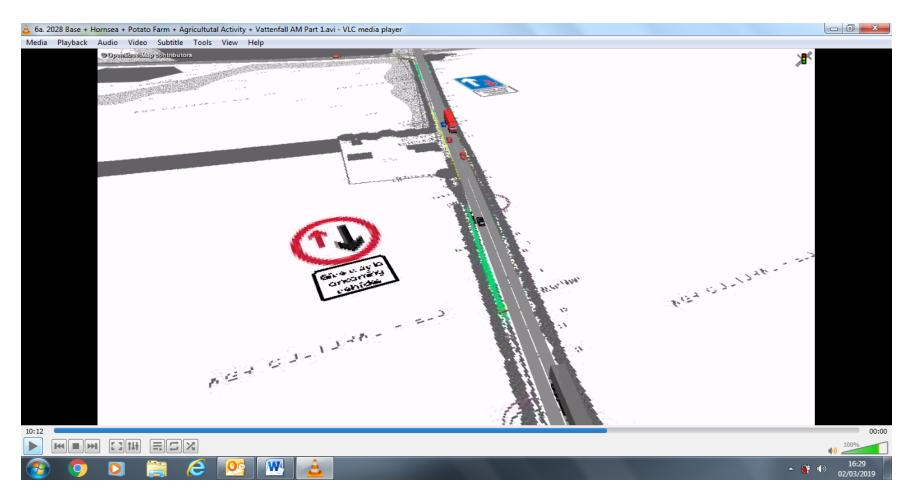
Priority signs not working at the hump: it is impossible for an HGV and a car to pass at that location.
